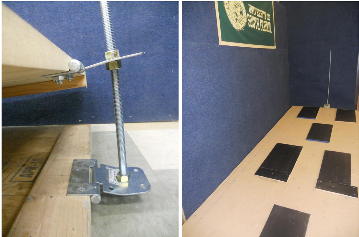
Figure 4.1: Ramp construction. Left: The ramp uses a power screw to lift the inclined portion. Hex nuts are used to lock it at a specific angle. Right: Tiles are used for extra foot clearance and to damp out unwanted vibration at foot impacts.
