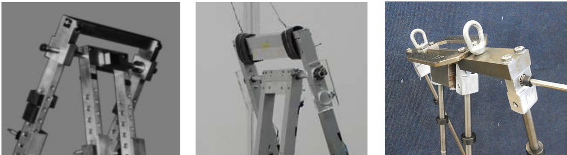
Figure 3.3: Comparison of several crossbar assemblies. Left to right: Garcia et. al crossbar [6], Trifonov et. al crossbar [11], and the current planar crossbar mechanism.
