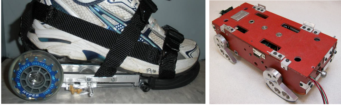
Figure 2.5: GEMS Shoe designs. The left shoe was developed by de Groot et. al [5] in 2009. This completely passive shoe uses a rack and pinion to convert the user's energy into a backwards motion. While the right shoe is also completely passive, it uses a magnetic particle brake to generate a more controlled motion.
