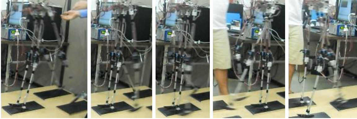
Figure 4.5: Foot clearance issue. Looking at the figure, the far outside leg enters the swing phase too soon causing it to catch on the first raised tile. Amazingly, the leg is able to continue through the swing phase and lock the knee. Even with this collision, the walker made it down the ramp.
