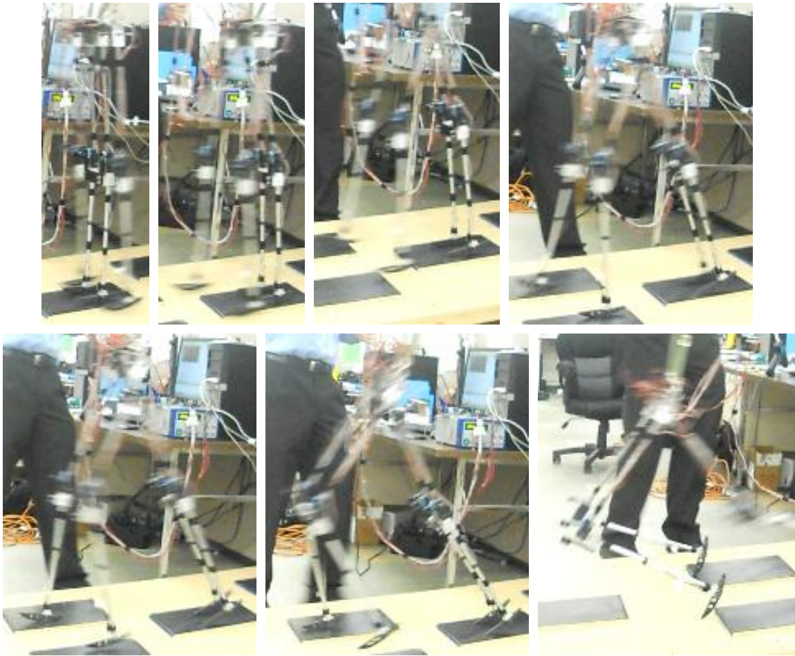
Figure 4.4: Loss of foot friction. As the walker made contact with the ramp tile at the second heel strike, each outer leg made contact separately. This imbalance caused the foot to bounce and skid.
