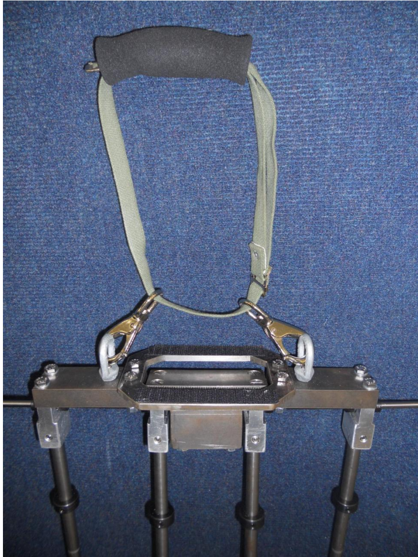
Figure C.1: PDW handle for walker testing. The handle is directly bolted to the crossbar and can be removed by two metal clips. It was constructed to decrease the likelihood of walker damage due to falls
